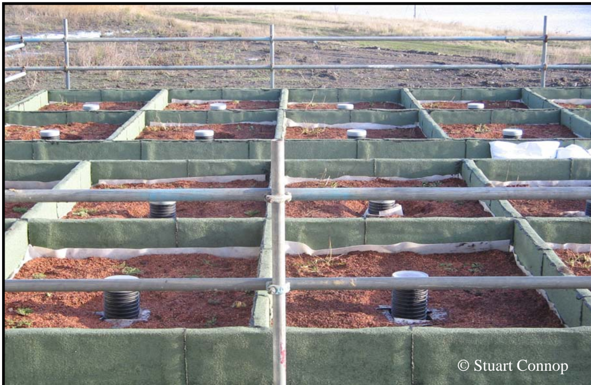
Figure 2. Green roof test platforms constructed at Barking Riverside offices.
